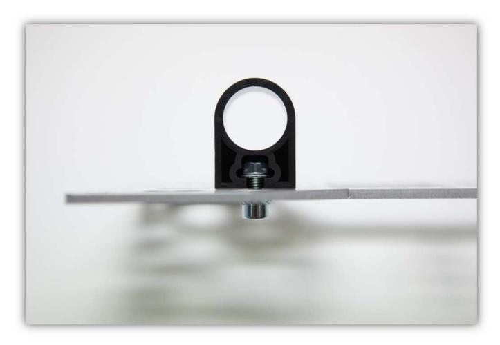
Repeat this 3 times in the positions shown on the pictures. Remember, do not fully tighten these bolts. Just hand tighten them.
