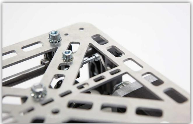
Tighten the bolt that holds the MICROSWITCH MOUNT in place.
