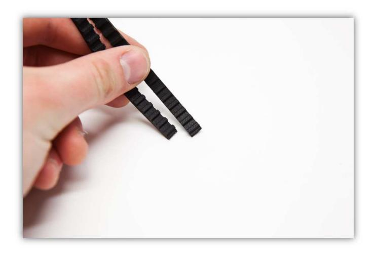
Now from the end you just cut, measure the belt for 63.5 cm (25") or 127 teeth. This measurement is critical. We advise to count the teeth and also measure the distance before cutting.
