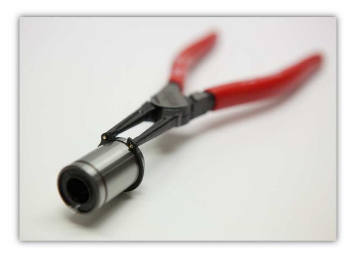
Slide the bearing with one circlip inside one of the BEARING CLAMP X pieces:
