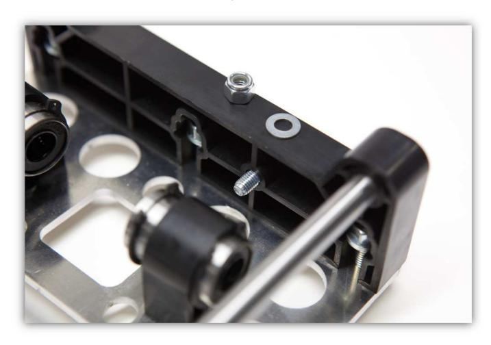
Place the small aluminium bracket as shown in the picture and tighten the assembly.
