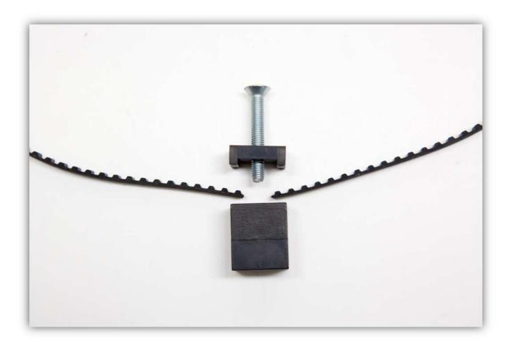
Assemble them as shown in the picture. Take notice that the belt sits between the clamps exactly as in the picture.
