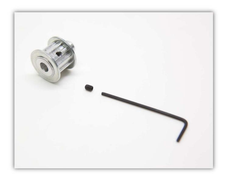
Screw the bolt into the pulley.
