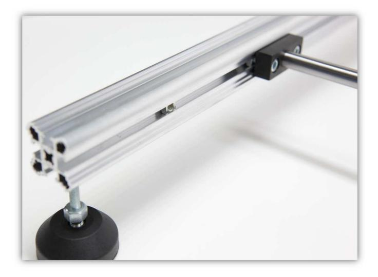
Slide the X carriage further until there is approx. 4 mm (0.16") between the first ROD CLAMP X piece and the ANGULAR MOUNT on the end of the frame. Make sure the X CARRIAGE is level and parallel inside the frame. Also check if the BEARING CLAMP X pieces are still in the right place. The bolts holding these pieces in place should still be just hand tightened.
