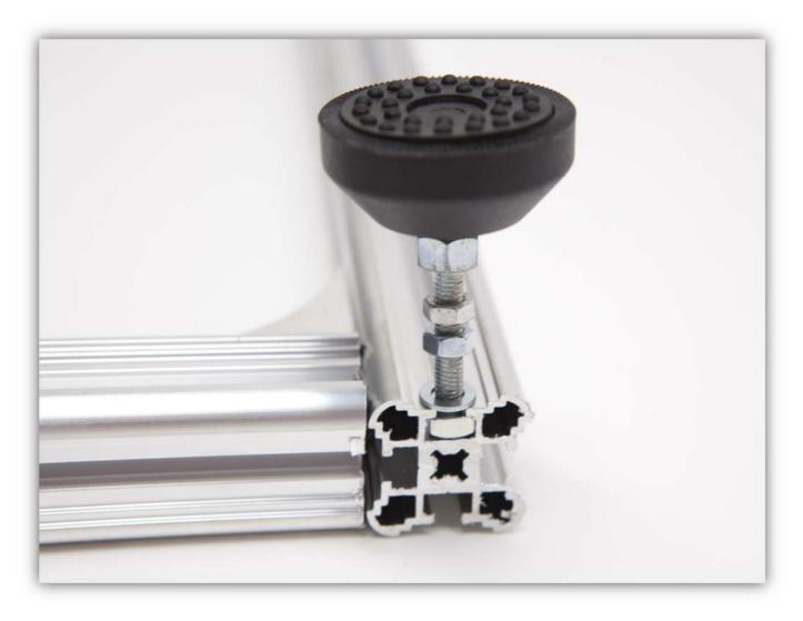
Tighten the nuts firmly as in the picture below:
