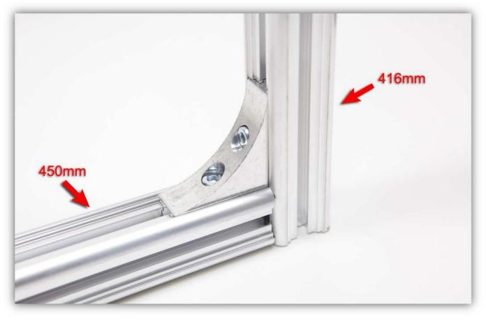
Tighten all the bolts firmly and make sure all angles are 90° and all ALUMINIUM PROFILES are flush.
