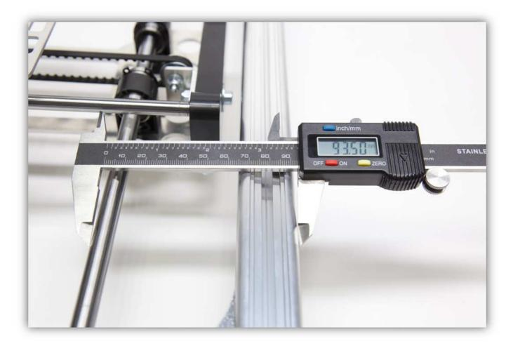
Now tighten the bolts on de ROD CLAMP X pieces securing the X carriage in place.
