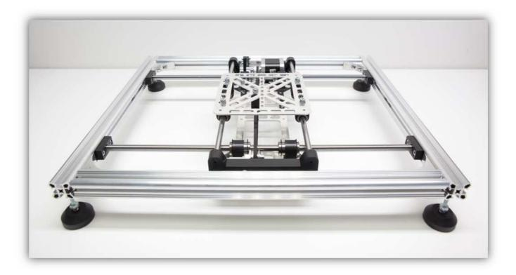
Make sure you have enough clearance between the BEARING CLAMP Y pieces and the LINEAR BEARINGS in the BEARING CLAMP X pieces. You can slide these bearings a few millimetres out of the way when there is not enough clearance. The 2 carriages should now move freely along the full length of all the rods.
