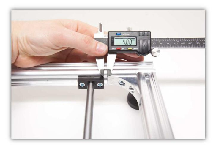
Now slide an ANGULAR MOUNT on each ALUMINIUM bar on the open side of the frame.
