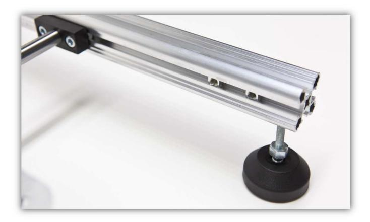
Slide one square M5 nut into the left ALUMINIUM PROFILE as shown:
