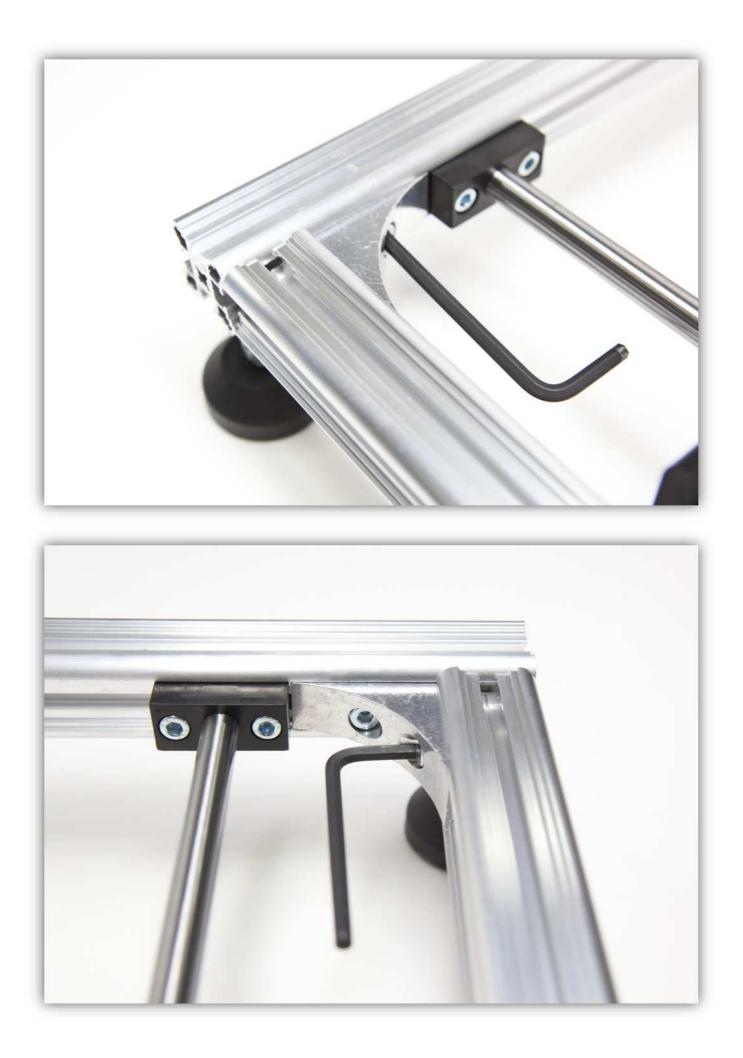
Now after making sure that the BEARING CLAMP X pieces are still in the right place, you can tighten these bolts holding them in place. Make sure the X CARRIAGE can move freely.
