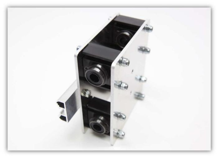
**Slightly** tighten the bolts. We will fully tighten these bolts at a later step in the building process.
