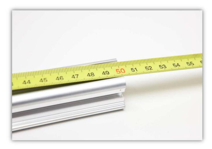
Slide two ANGULAR MOUNTS (from the box) in the end of the ALUMINIUM PROFILE of 500 mm (19.7").
