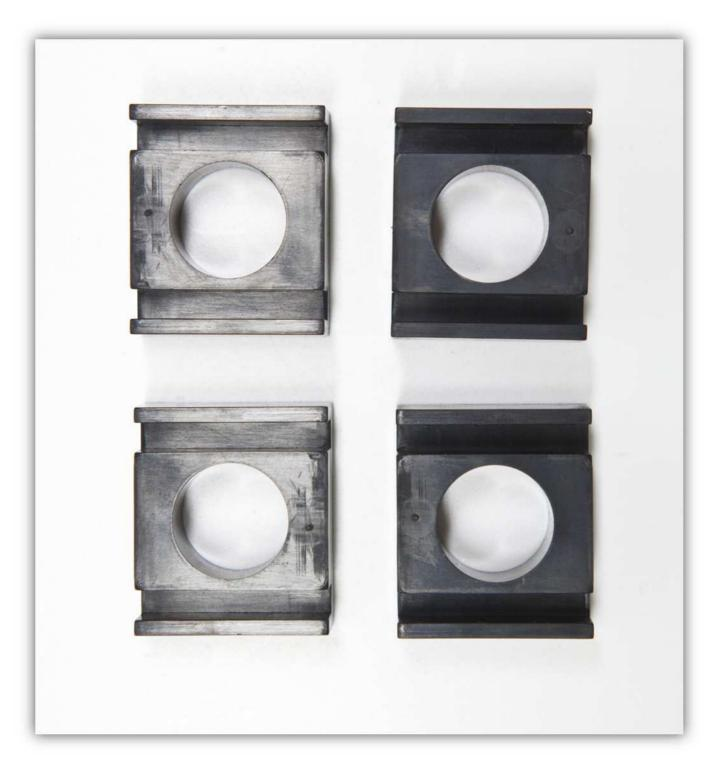
Slide 4 linear bearings into the 4 BEARING CLAMP Z BIG pieces.
