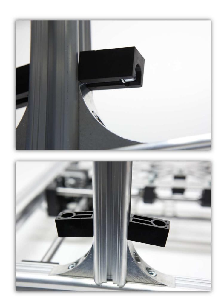
Make sure that the ROD CLAMP Z BIG pieces are as far down as possible and then tighten the bolt. **Do not over tighten this bolt.**
