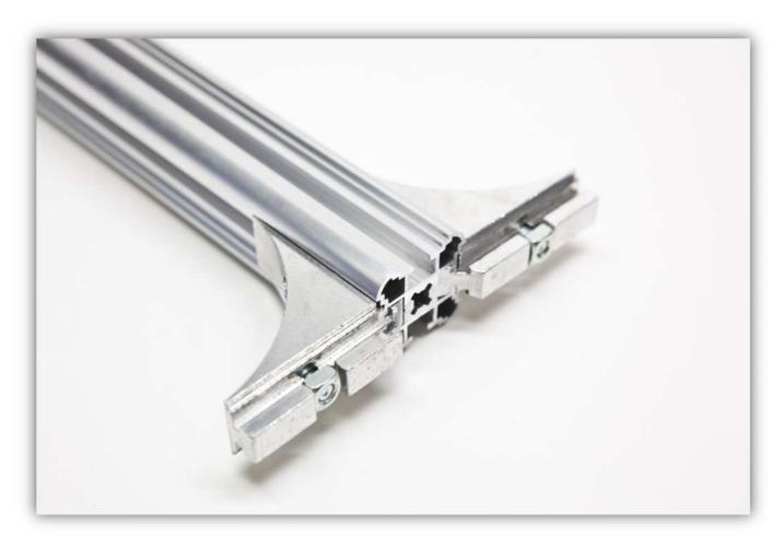
Slide this assembly in the left profile of the BASE FRAME.
