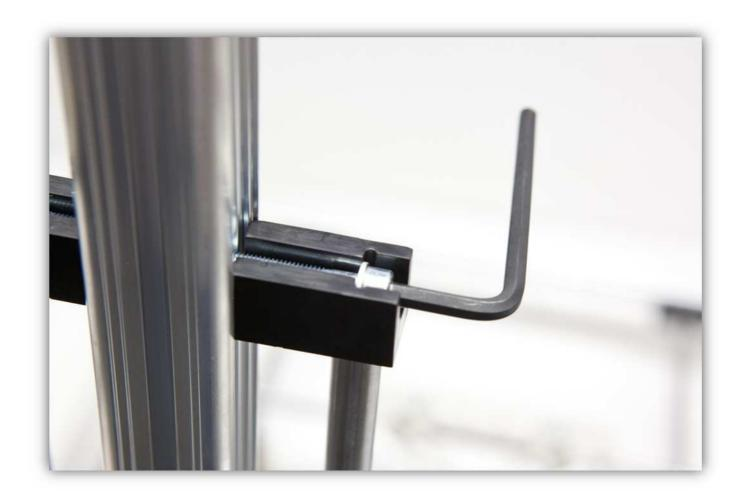
Making sure that this Z CARRIAGE can move freely up and down, you can firmly tighten all the bolts that were previously only slightly tightened.
