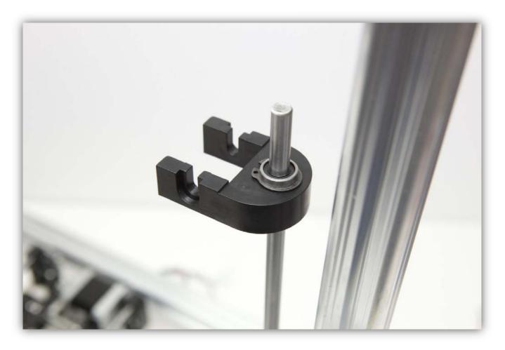
Slide one of the M5 bolts (with washer and square nut) and slide it down the ALUMINIUM PROFILE and slide a ROD CLAMP Z SMALL over this bolt. It should fit over the rod.
