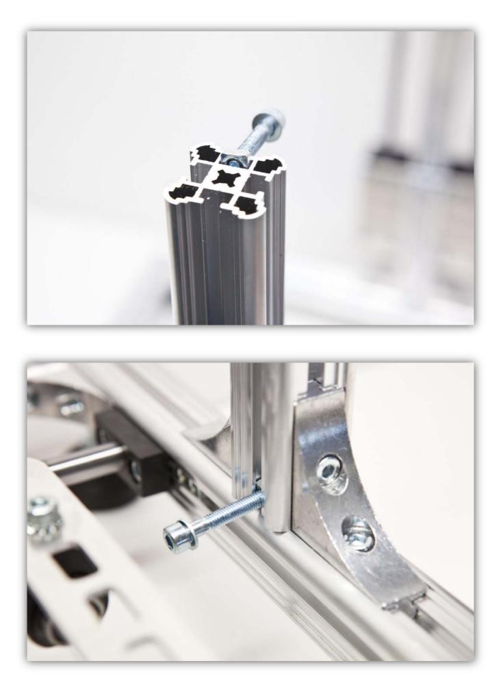
Slide one of the ROD CLAMP Z SMALL pieces over this bolt and make sure you tighten this bolt so that this piece sits at about 6 cm (2.36") of the base frame.
