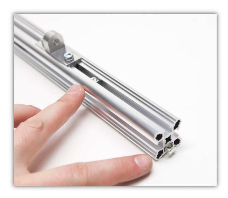
Now slide the ALUMINIUM PROFILE into the BEARING CLAMP Z SMALL piece.
