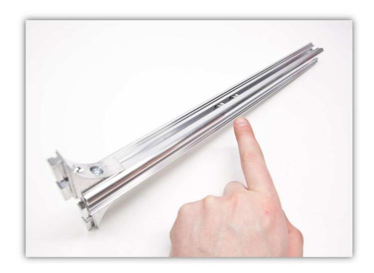
Slide the FAN HOLDER BRACKET and 1 square M5 nut into the ALUMINIUM PROFILE. **Notice the orientation of each part.**
