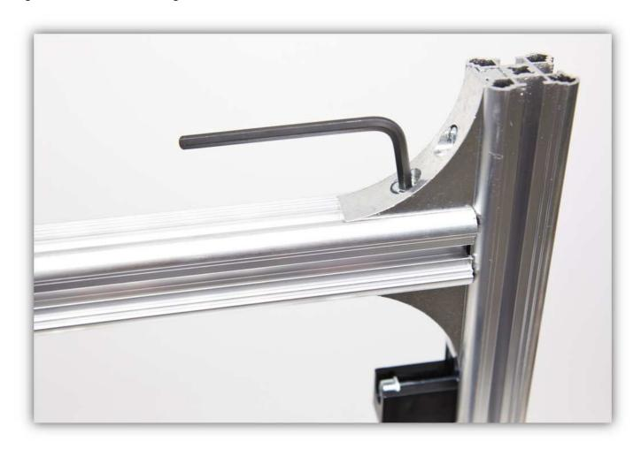
Slide the two square nuts on the opposite of each other in the extruder arm towards the BEARING CLAMP Z SMALL piece.
