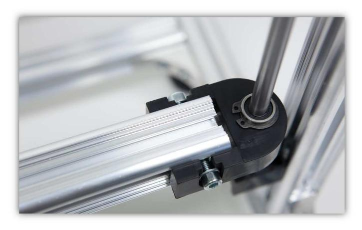
Tighten these bolts while making sure the Z CARRIAGE and the EXTRUDER ARM move freely.
