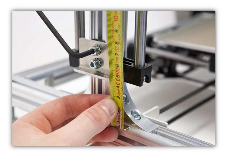
Take the 2 M3 bolts and 2 M3 toothed washers and bolt the motor to the bracket.
