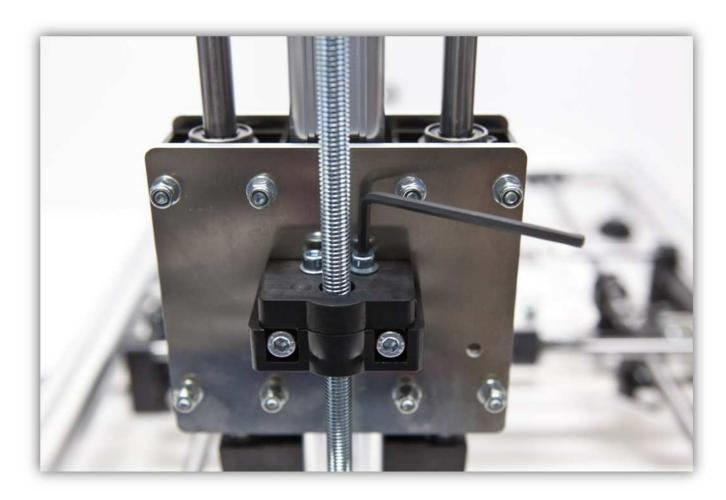
Now fully tighten the bolts that attach the Z FOLLOWER assembly to Z CARRIAGE assembly.
