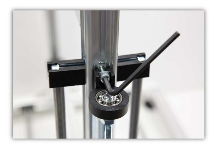
Slide this bolt and Z ROD GUIDE down until the 608 bearing meets the M8 washer.
