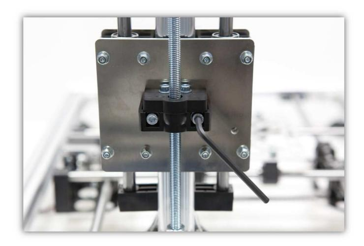
Screw an M8 locking bolt on the rod followed by an M8 washer.
