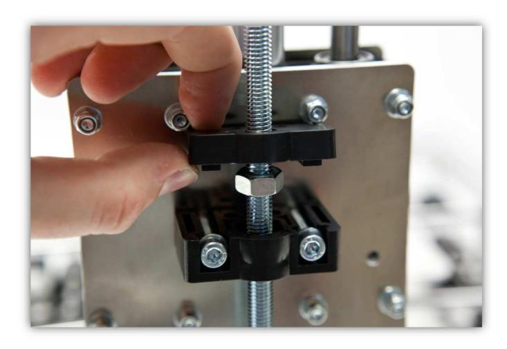
Tighten the MOTOR CONNECTOR to make sure there is no play.
