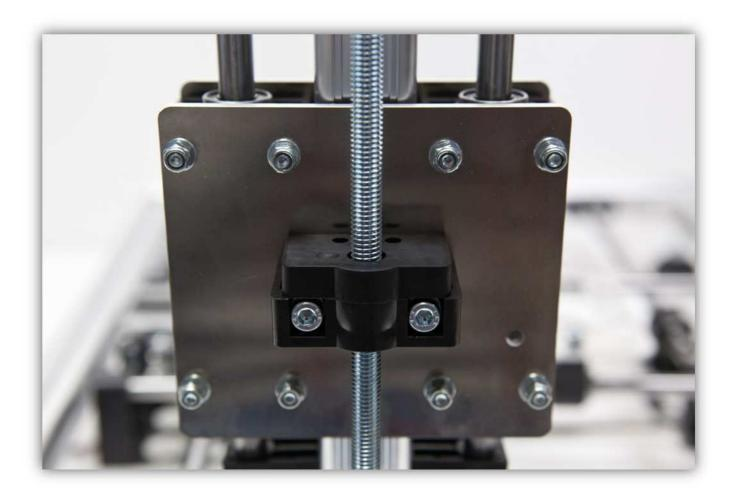
Take the 2 M4 bolts and 2 M4 washers and screw them into the top of the Z FOLLOWER assembly as shown in the picture below.
