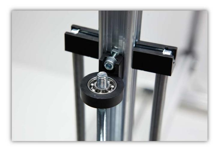
Screw an M8 locking nut over the rod as shown in the picture.
