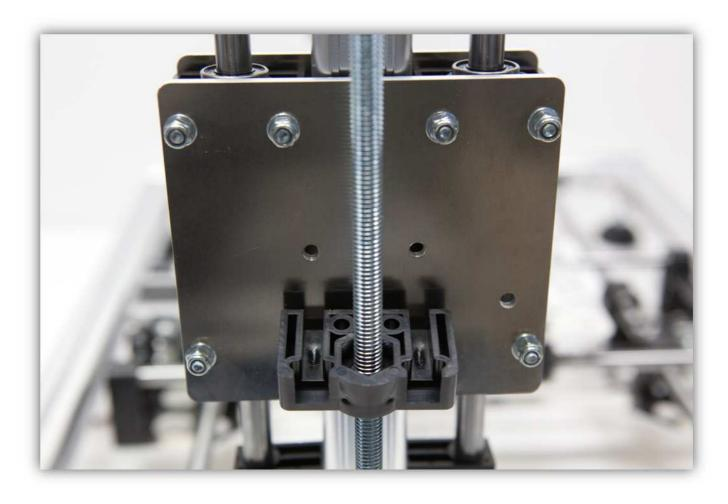
Screw the M8 nut over the rod and take the 2 M5 bolts and 2 M5 washers and screw them into the Z CARRIAGE.
