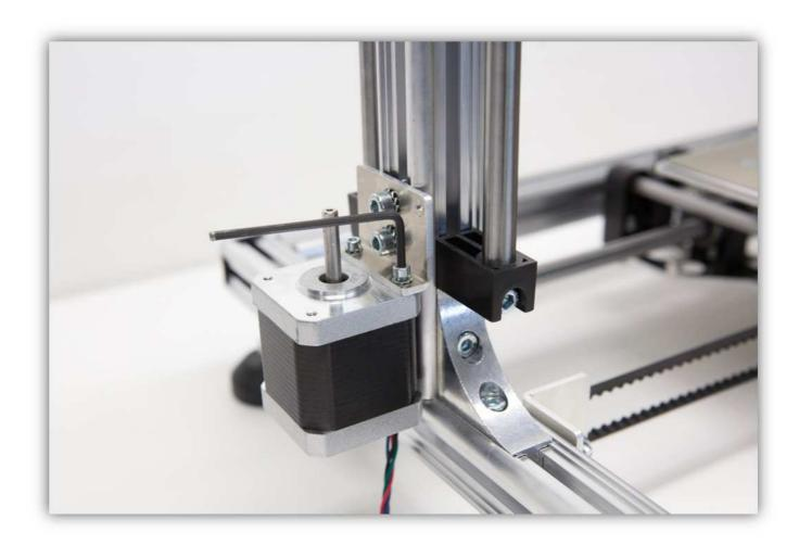
Screw an M8 bolt followed by an M8 washer, an M8 toothed washer, an M8 washer and the MOTOR CONNECTOR as shown in the picture below.
