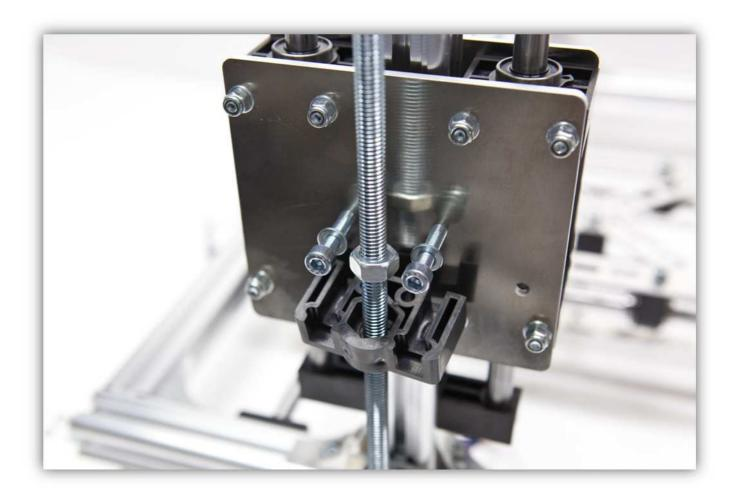
Slide the Z FOLLOWER B piece over the rod as shown in the picture. Watch the orientation.
