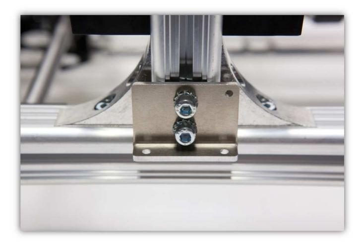
Make sure the bracket bottom is at **MAXIMUM** 4.5 cm (1.77") from the bottom frame. It should be between 4 cm (1.57") and 4.5 cm (1.77"). Tighten the 2 bolts and **make sure that the bracket is perfectly horizontal.**
