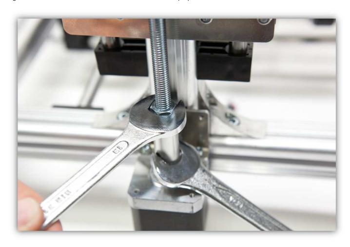
Attach the Z FOLLOWER A piece to the CARRIAGE. **Do not fully tighten these bolts.** Turn the rod until the M8 bolt sits snugly into the Z FOLLOWER A piece.
