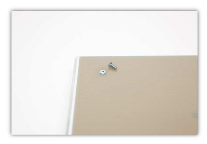
Use 4 M3 washers and 4 M3 nuts to secure the HEATED BED PCB to the BED PLATE.
