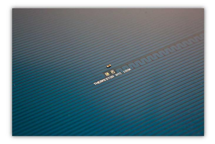
Place the NTC THERMISTOR with one side on the pad while you apply heat, it does not matter which side, a thermistor is not polarized. **Make sure you do not heat the thermistor for too long.**
