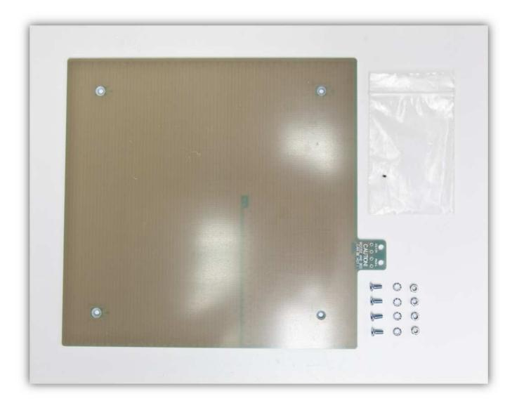
Lay the CARDBOARD ISOLATOR on top of the BED PLATE and align the holes. Watch the orientation of the bedplate carefully.
