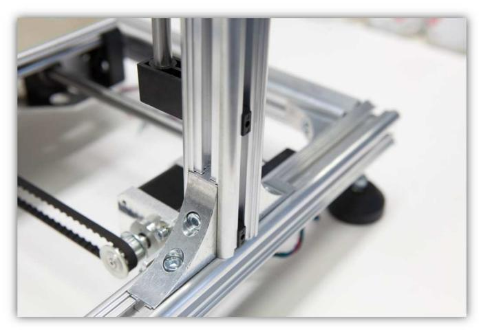
Next slide the COIL SUPPORT in the same profile and align it with the horizontal ALUMINIUM PROFILE. Tighten it firmly.
