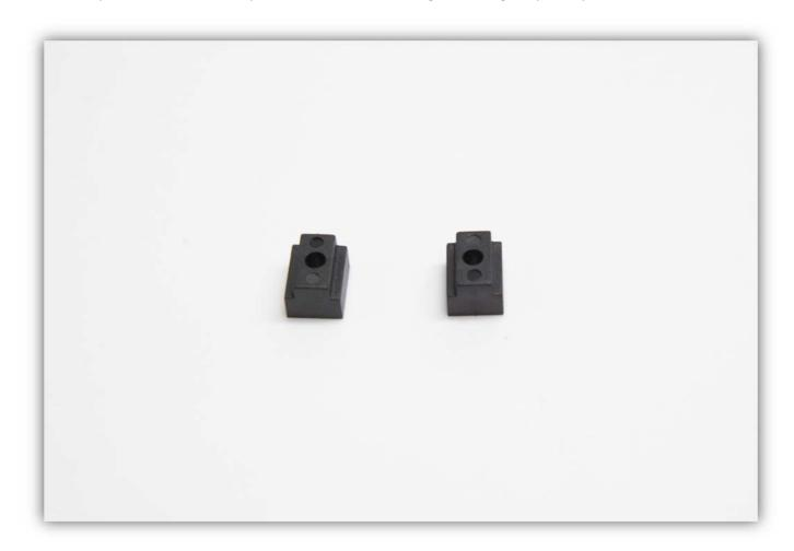
Slide these PROFILE MOUNTS in the right upright ALUMINIUM PROFILE as shown in the pictures below.
