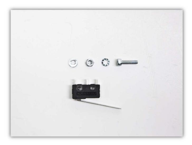
Slide the M3 bolt with an M3 washer and an M3 toothed washer through the micro switch as shown in the pictures.
