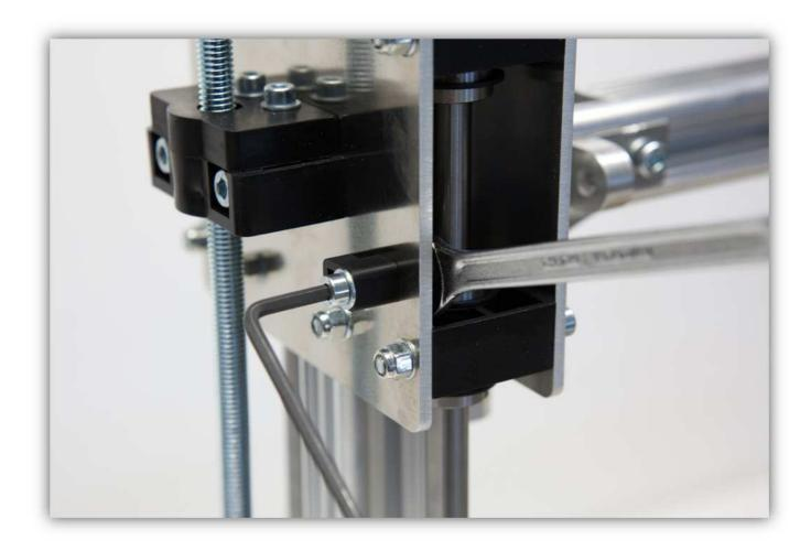
Use the long M3 screw with an M3 nut and an M3 toothed washer as shown in the picture.
