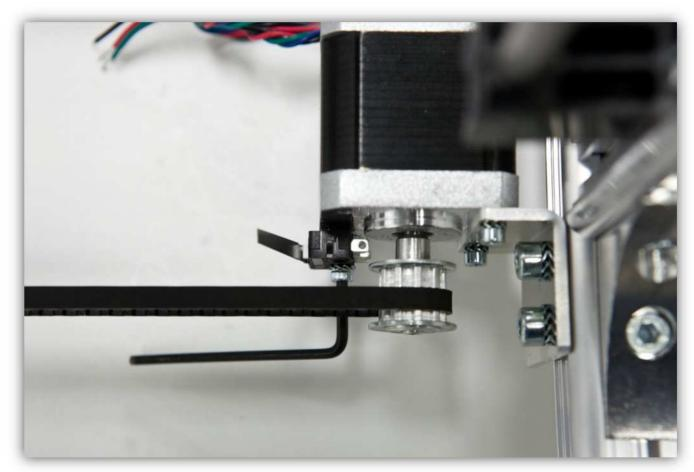
Make sure that the micro switch is in line with the screw on the X CARRIAGE. If not you will have to reposition both X PULLEY BRACKET and X MOTOR BRACKET.
