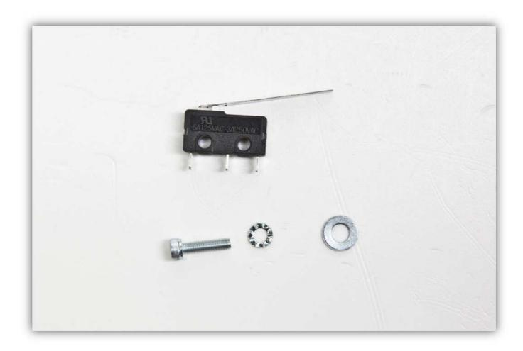
Slide the M3 bolt with an M3 toothed washer through the micro switch. \\
