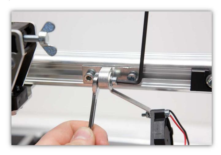
Tighten the bolt on the fan, make sure that the fan is level.
