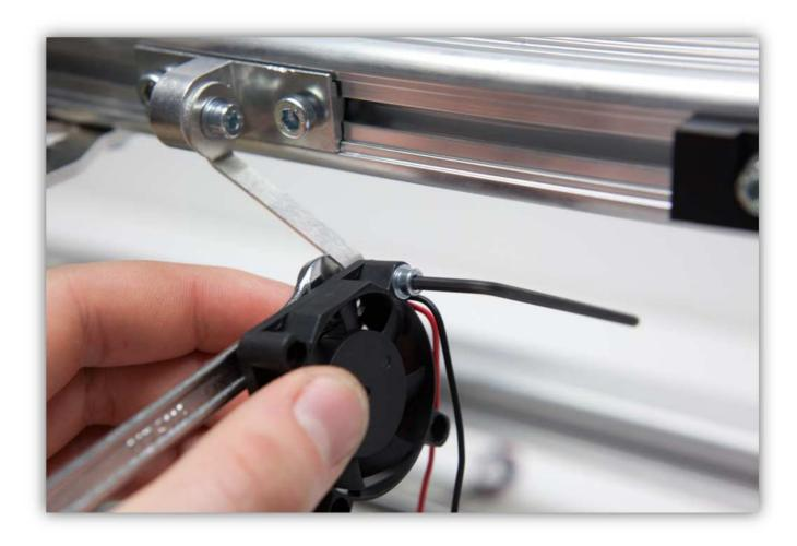
Slide the FAN HOLDER BRACKET closer to the extruder and tighten it firmly.
