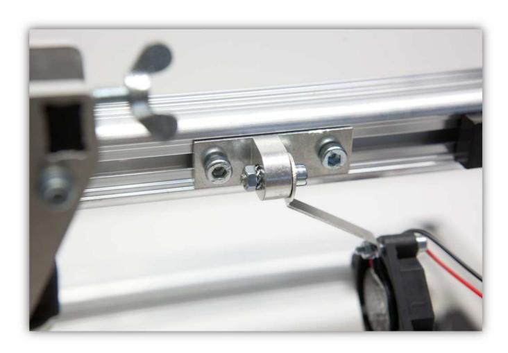
Tighten this bolt, make sure that the FAN HOLDER is vertical.
