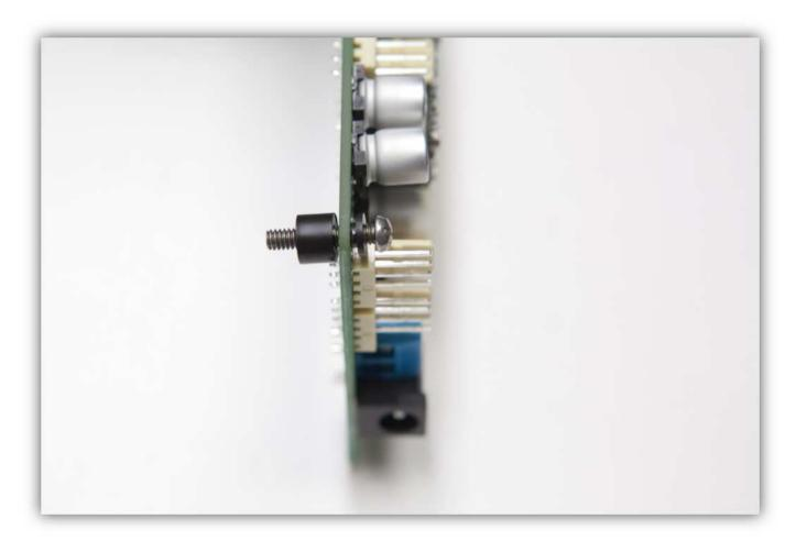
Screw the bolts into the PROFILE MOUNTS.
