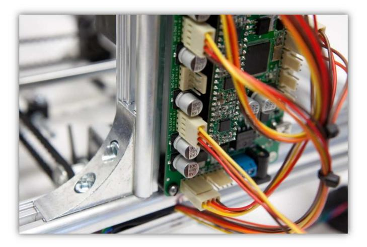
Cut the wires of the X axis motor down to about 15 cm (5,9").
