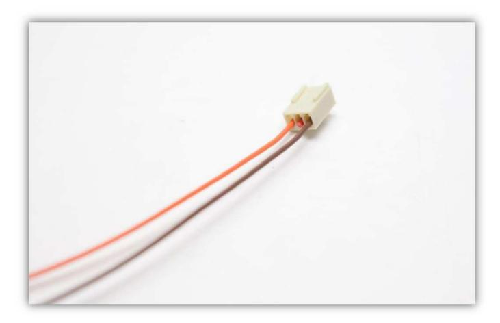
Plug the female connector in the male connector labelled with XSTOP on the controller board.
