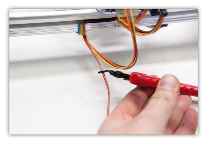
Strip 5 mm (0.2") and tin the ends of these wires.
