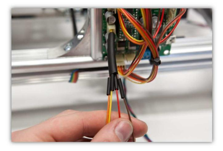
Solder the 4 wires from the motor to the 4 wires of the connector you tinned earlier. Watch the colours closely.
