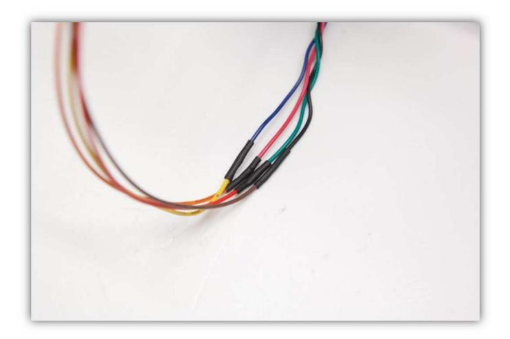
Now slide the big piece of heat shrink tubing over the 4 small pieces, heat the big piece so it covers and protects the 4 heat shrunk joints.
