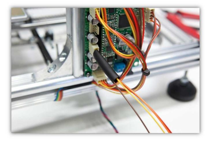
Slide the 4 small heat shrink tubes over the 4 wires of the connector.
