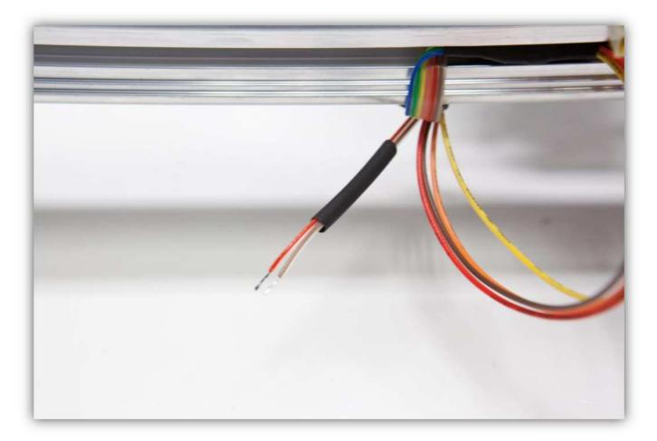
Slide the 2 small heat shrink tubes over the 2 wires of the connector.
