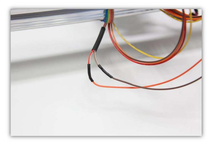
Now slide the medium size piece of heat shrink tubing over the 2 small pieces, heat the medium size piece so it covers and protects the 2 heat shrunk joints.
