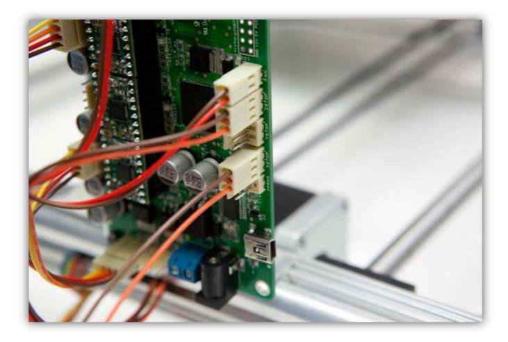
Cut the **Red** and **Brown** wire from the X micro switch so that it can connect to the wires of the connector you just plugged in.
