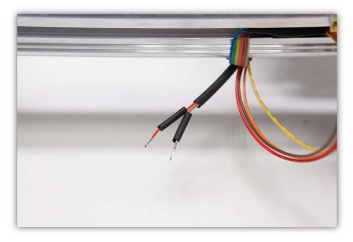
Solder the 2 wires from the **Red** and **Brown** wire to the 2 wires of the flat connector you tinned earlier. **Watch the** colours closely.
