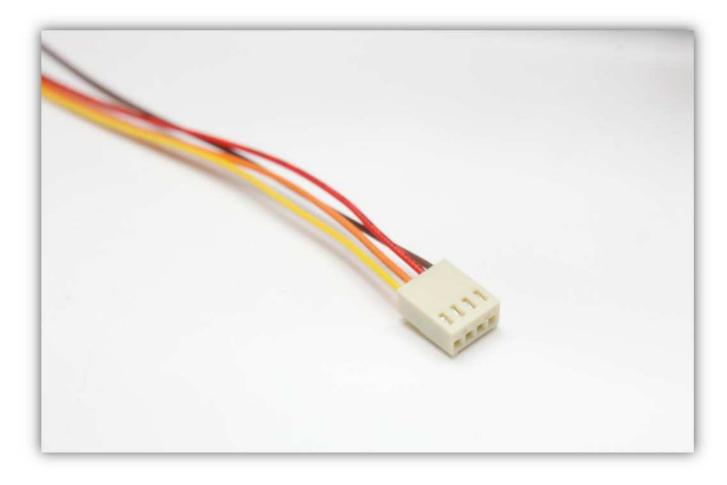
Plug the female connector in the male connector labelled with X-MOTOR on the controller board.
