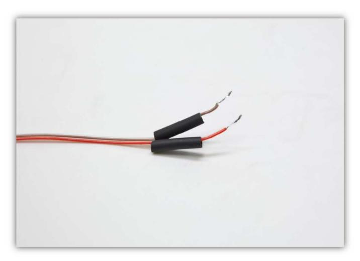
Solder the wires to the contact points of the micro switch, slide the heat shrink tubes over the contacts and shrink them.
