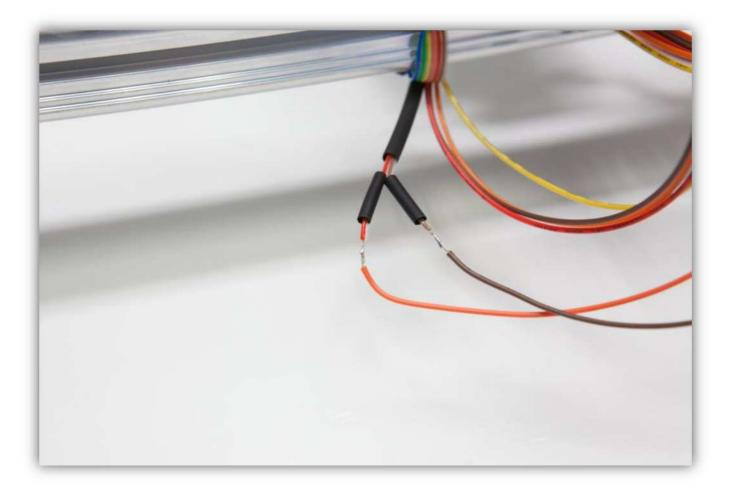
Slide the 2 small heat shrink tubes over the solder joints and heat them up.
