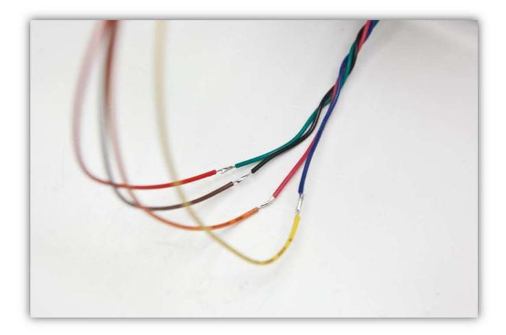
Slide the small heat shrink tubes over the solder joints and heat them up so they shrink.
