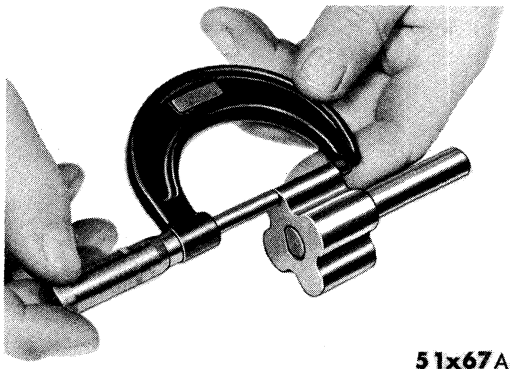
Fig. 92 — Measuring Inner Rotor Thickness
