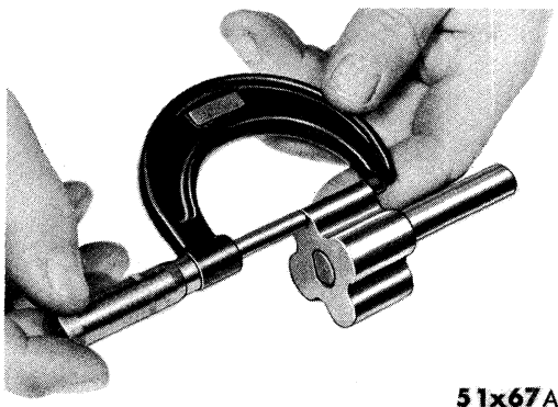
Fig. 92 — Measuring Inner Rotor Thickness
