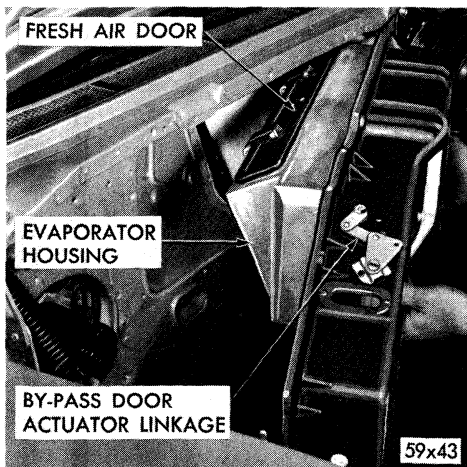
Fig. 145 — Removing or Installing Evaporator Assembly
