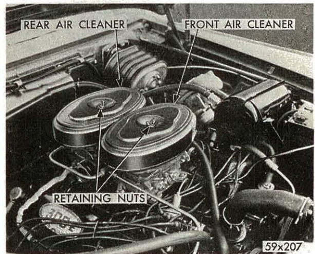
Fig. 6 - Carburetor Air Cleaners Installed
