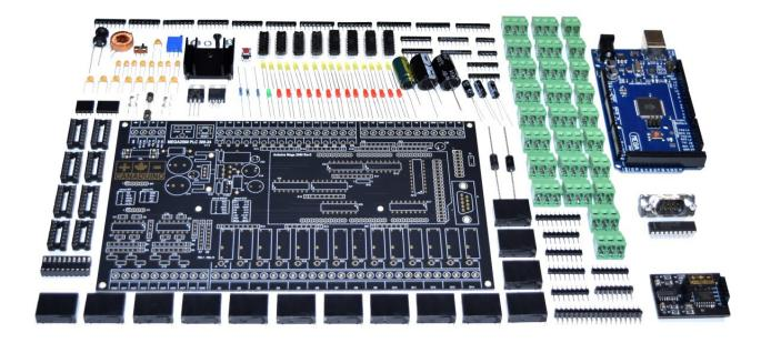
DIY Kit with all included parts. Arduino module, SD-Card + RTC module, and MAX233CPP serial chip are sold separately.
